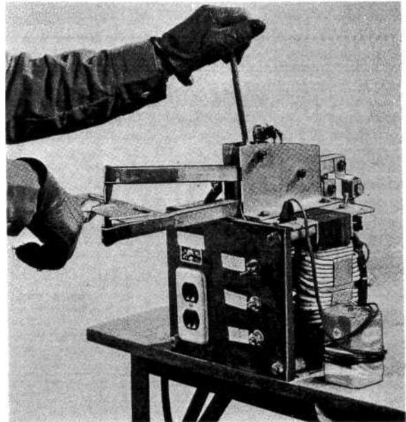
Switches and taps on insulating panel should be labeled for easy identification and to prevent error. Do this with masking tape and a pen
