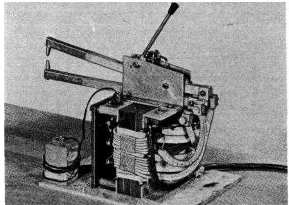
A 6-V. battery provides automatic operation of the relay. Relay also can be operated manually. Drawing below shows the wiring diagram of welding unit
